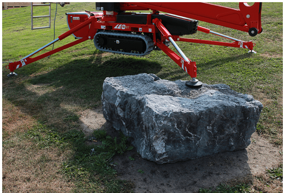
Can be jacked up on ground slopes up to 10,0 ° / 17,5 %
