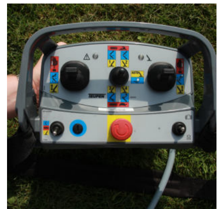
User-friendly cable control with colour coded functions
