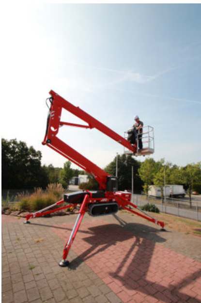
Automatic self-levelling stabiliser system
